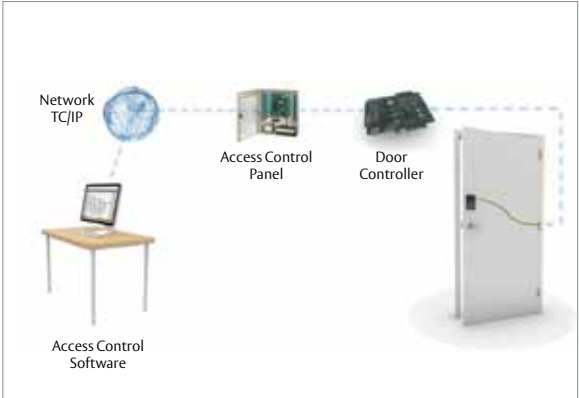
Typical Integrated Wiegand Configuration
