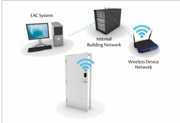
Typical WiFi System Configuration
